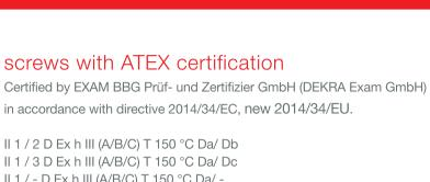
II 1 / 2 D Ex h III (A/B/C) T 150 °C Da/ Db II 1 / 3 D Ex h III (A/B/C) T 150 °C Da/ Dc II 1 / - D Ex h III (A/B/C) T 150 °C Da/ -
